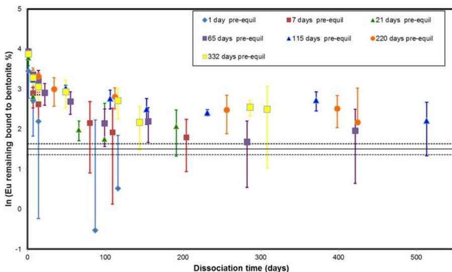
FIG. 1. Natural log of percentage of Eu bound to bentonite vs. EDTA contact time, as a function of pre-equilibration time (pH =  $7 \pm 0.1$ ; I = 0.1 M NaClO<sub>4</sub>). The full black horizontal line represents the equilibrium position, and the dashed lines represent the experimental uncertainty for the equilibrium position. Errors bars are  $2\sigma$  based on the standard deviation of triplicate measurements.
