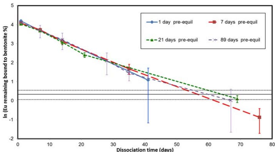
FIG. 3. Natural log plot of the colloid dissociation experiment:  $\ln(\text{percentage bound to bentonite})$  vs. Dowex resin contact times, as a function of pre-equilibration time ( $\text{pH} = 8.8 \pm 0.1$ ). The black horizontal line represents the equilibrium distribution, and the dashed lines represent the experimental uncertainty ( $1.4 \pm 1.1\%$ ).
