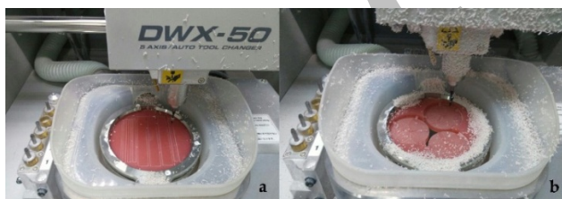
Figure 1: Showing CNC milling machining. (a) for Impact, Flexural & (b) for Surface roughness Group II Specimens.
