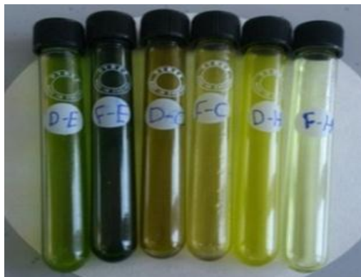
Figure 1: Picture shown fresh and dry leaves Soxhlet extracts (DE: Dryethanol, FE: Fresh ethanol, DC: drychloroform, FC: freshchloroform, DH: Dry hexane and FH: Fresh hexane).
