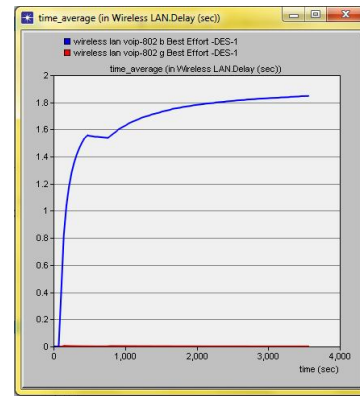
Figure 11: Wireless LAN delay for IEEE802.11b and IEEE802.11g with best effort service
