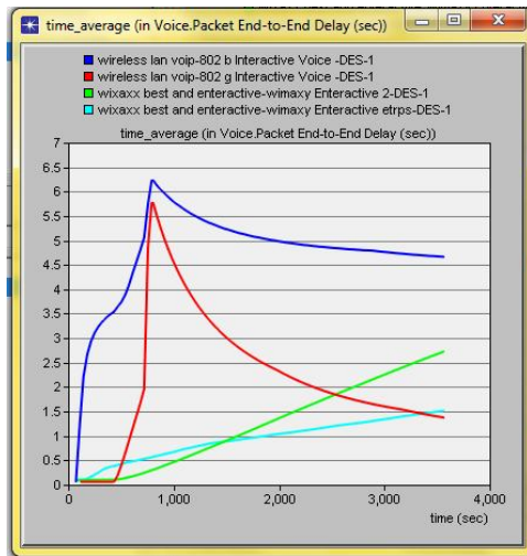
Figure 24: Voice packet end-to-end delay on Wi-Fi and WiMAX networks with interactive service
